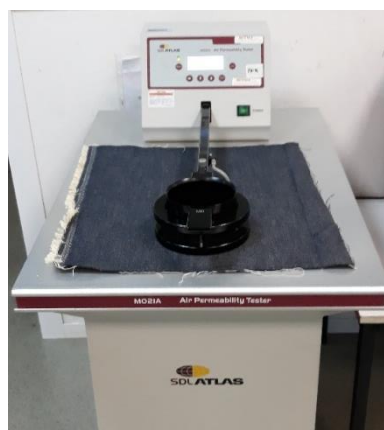
Figure 3. Air permeability measurement
