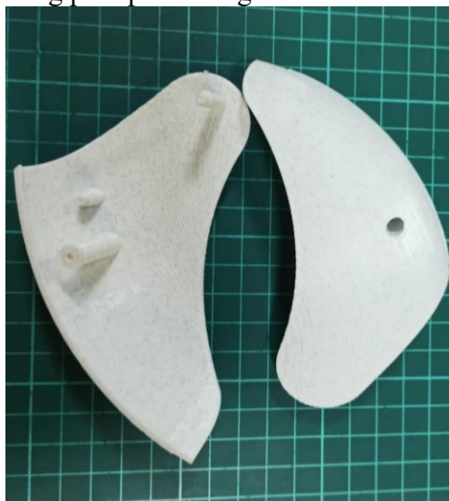
Figure 4 3D Print of shoulder's plastic apparatus
