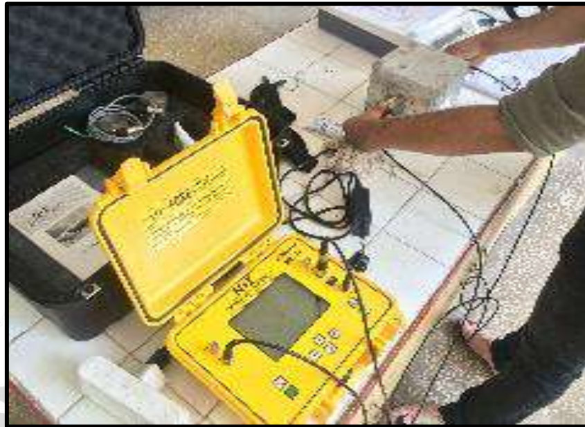
Figure 2. Ultrasonic Pulse Velocity test device
