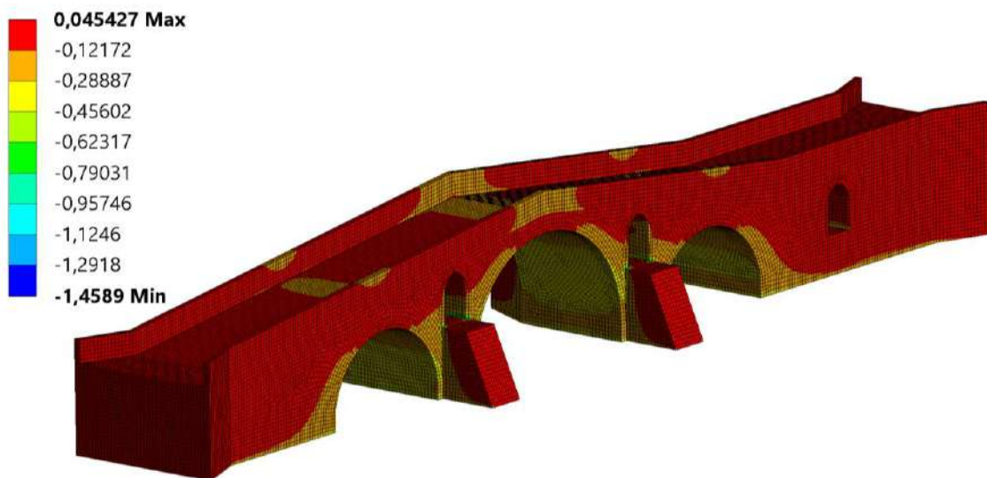
Fig. 6. Minimum principal stress obtained from the static analysis
