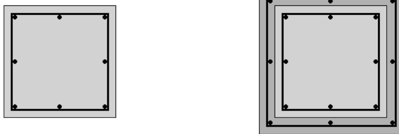
Figure 2. Jacket Application on Columns
