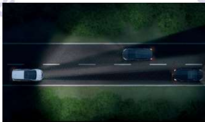
Fig. 11: Automatically adjust the illumination of the road to the traffic situation [11]
