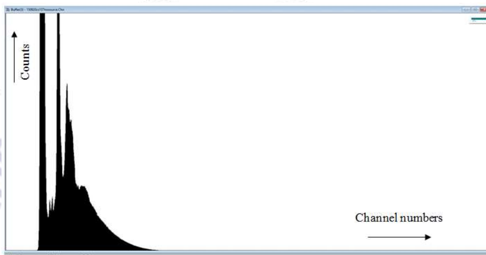
Figure 4. MPPC module output spectrum without gamma source (MCA screen view).
