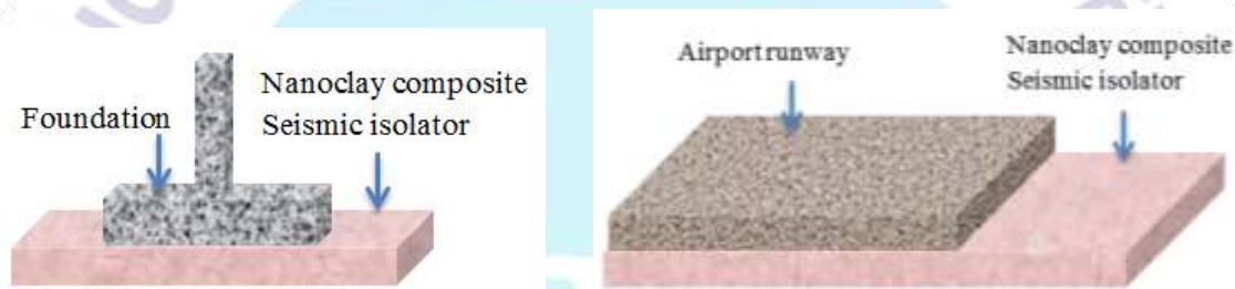
Figure 18. Possible applications of nanoclay composite based seismic isolator
