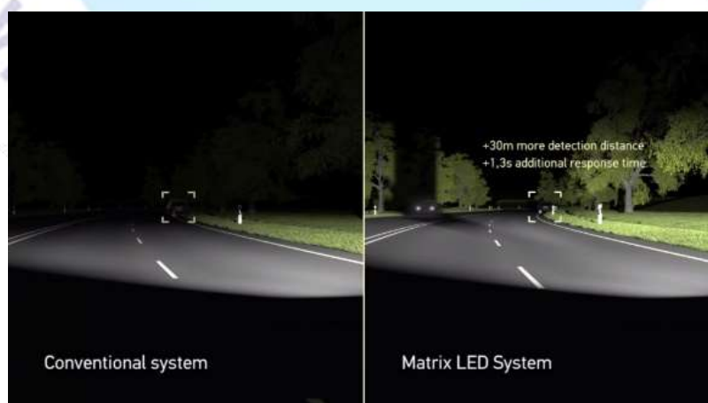
Fig. 6: Comparison of Conventional and Matrix LED for any object on the road [1]
