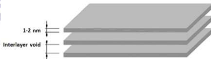
Figure 8. The structure of montmorillonite clay layers (Hollaway and Hackman, 2005)
