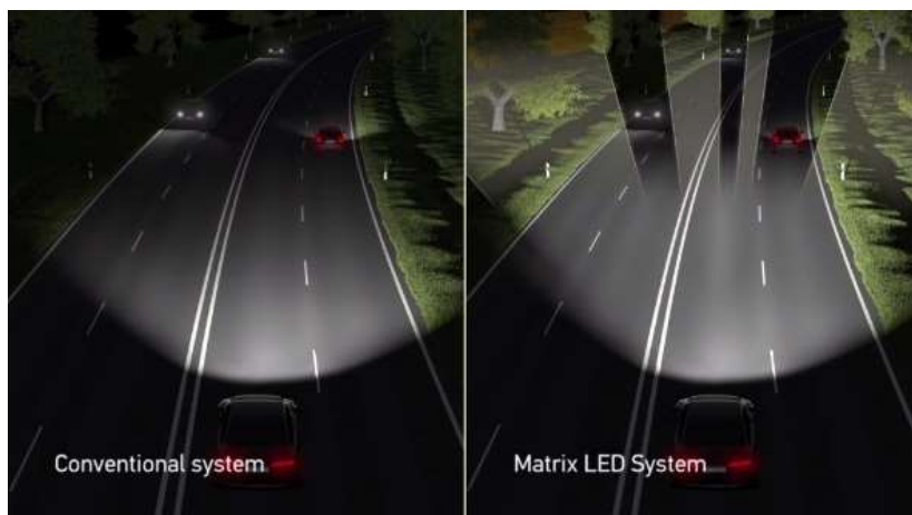
Fig. 7: Comparison of Conventional and Matrix LED for oncoming vehicle [1]
