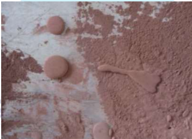
Figure 13. Water drops on the hydrophobic clay with modified DAMS (Kurt, 2009)
